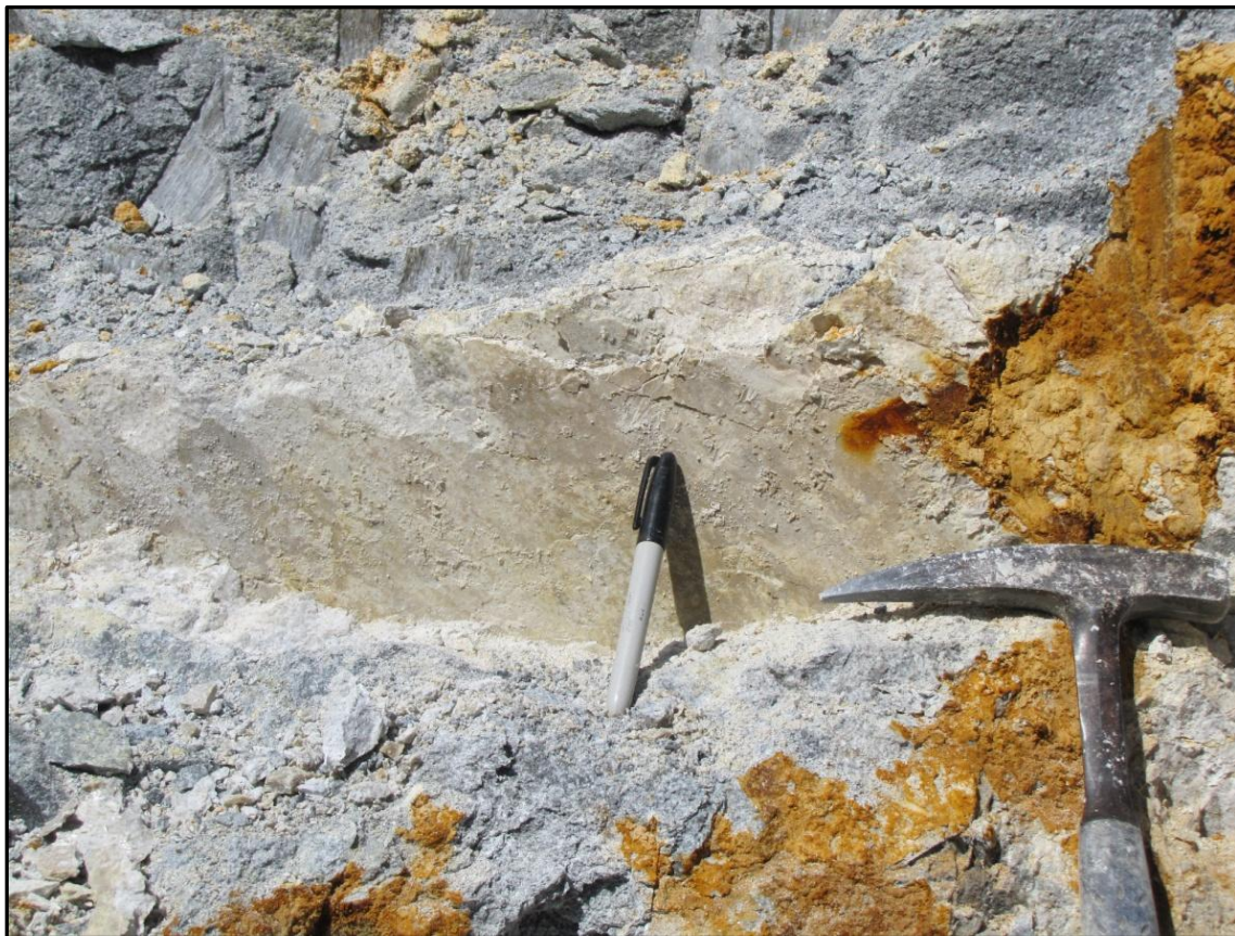
Figure 3.12. Fault zone slickenside. Picture of slickensides from the Open Pit white clay zones associated with faulting.
