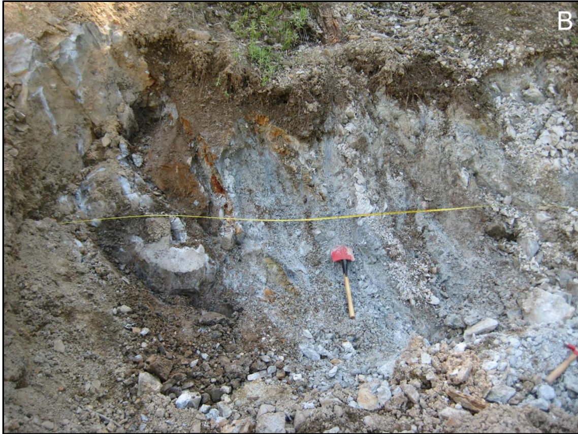
Figure 2.6. Road cut sampling site. (A) Clay zone SW of Foster Creek associated with a fault. (B) Excavation of surface layers covering the blue clay zone, exposing a > 5 m clay zone for sampling.
