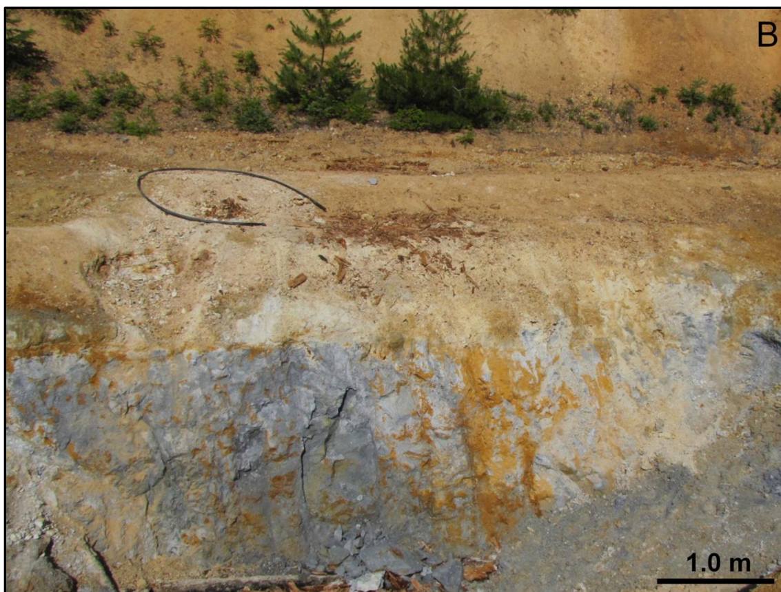
Figure 2.3. Open pit mine sampling site. (A and B) Open pit field area showing red-white oxidized clay zones above the un-oxidized blue clays. Solid white lines indicate the upper limit of the red and white oxidized zones, which are covered by glacial till. A series of NW-SE faults are present throughout the deposit, and exposed in the pit. (B) Image of the white-red oxidized zone with reduced blue clay zone beneath.
